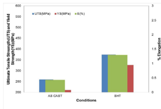
Fig. 1 (a) Ultimate tensile strength (UTS-MPa), 0.2% proof yields strength and % elongation for the as cast and SHT conditions
