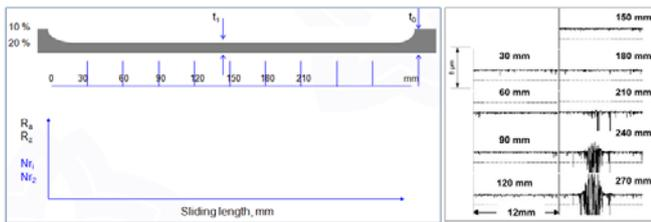
Fig. 4 Typical measurement of roughness profiles across the strip width at regular intervals,  $N_{r1}$ : Number of valleys deeper than 1.0  $\mu\text{m}$ ,  $N_{r2}$ : Number of valleys deeper than 2.0  $\mu\text{m}$
