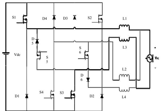
Fig. 2 Active stage of positive half line cycle
