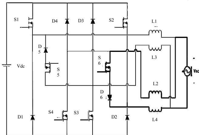
Fig. 5 Freewheeling stage of negative half line cycle
