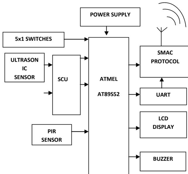
Fig.1. Block Diagram of Train 1 Section
