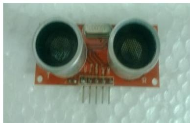
Fig.5. Image of Ultrasonic Sensor
