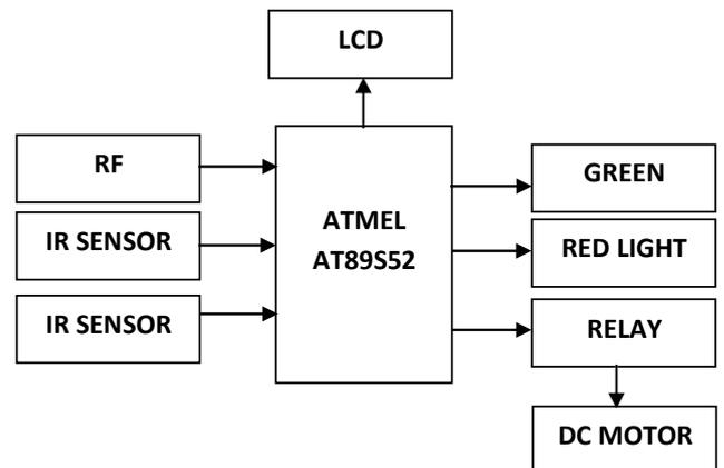
Fig.3. Block Diagram of Gate Section
