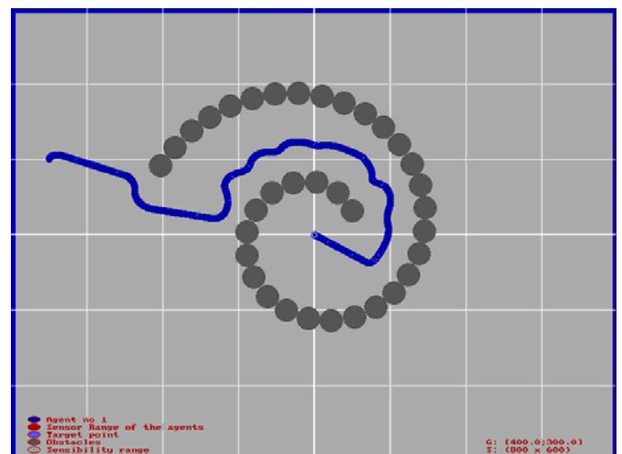
Fig. 9: A robot is trying to move toward the inner point of spiral.
