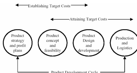
Fig. 3 Target costing and product development cycle. Ansari S., and J. Bell, (1996)
