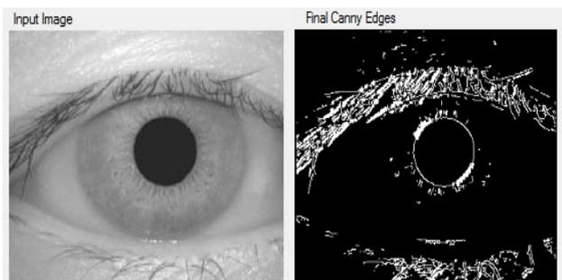
Fig. 8 Final Edges – Hysteresis thresholding by TH=40, TL=20
