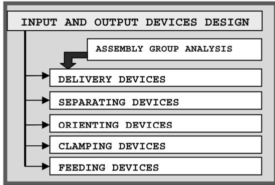
Fig. 5 Methodology of input and output devices design
