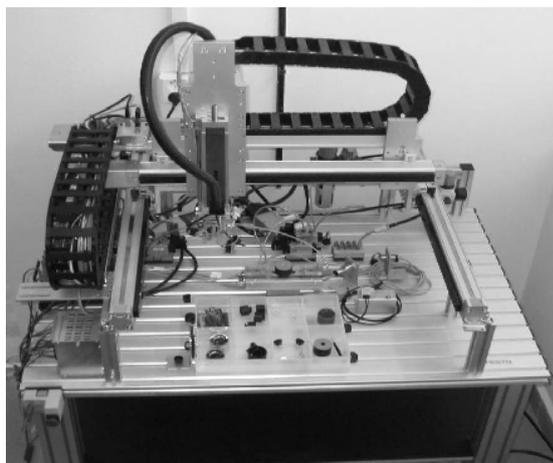
Fig. 11 Model of Cartesian robot for assembly and disassembly process
