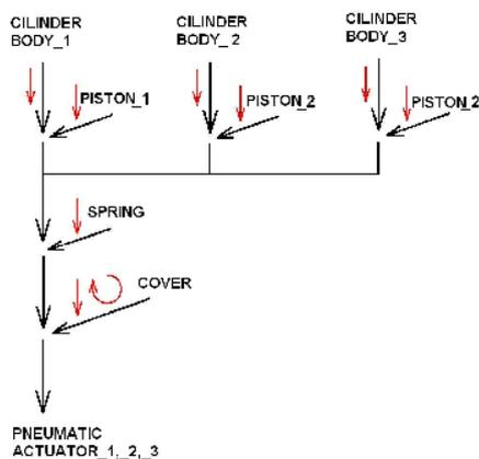
Fig. 8 Step diagram for assembly of pneumatic actuator
