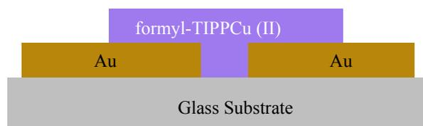
Fig. 2 Cross-sectional view of the Au/formyl-TIPPCu(II)/Au organic sensor
