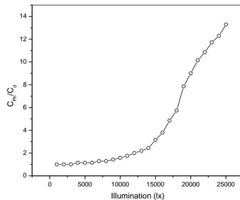
Fig. 5 Capacitance- illumination relationship for the Au/formyl-TIPPCu(II)/Au organic sensor.
