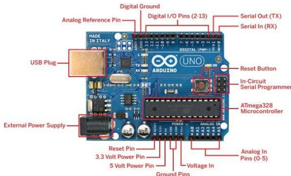
Fig. 1: Components in the Arduino board.
