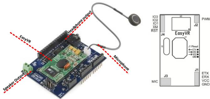
Fig. 2: Sound recognition module for Arduino.
