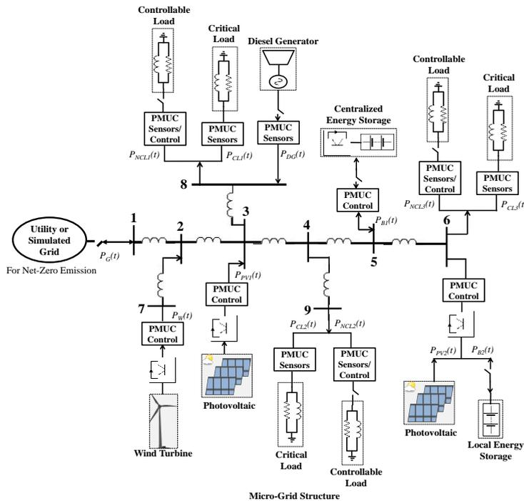
Fig. 3: 100kW micro-grid laboratory under development at Clemson University (under development).
