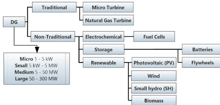
Fig. 1: Distributed generation types, technologies and sizes [14].
