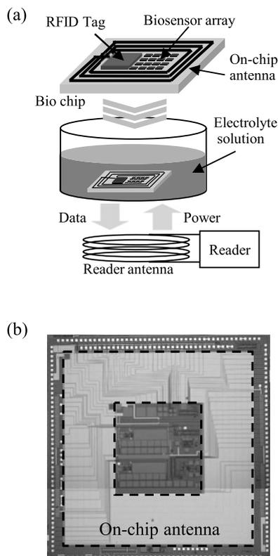
Fig. 1 (a) RFID biosensor measuring system.
