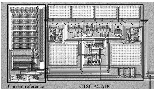
Fig. 7 Micrograph of CTSC  $\Delta\Sigma$  ADC.
