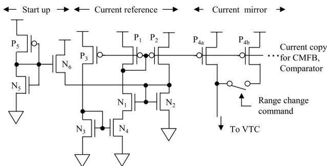
Fig. 3 Current reference with CMOS technology only.
