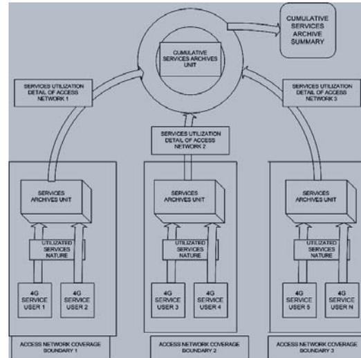
Fig. 2 Dataflow Diagram of Proposed 4G QoS Architecture
