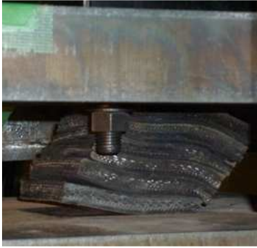
Fig. 6 Deformed STRP-6 at 103% lateral deformation
