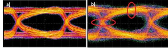
Fig. 3: Eye diagrams of received CPRI 3 with (a) and without (b) pilot tone transmission.
