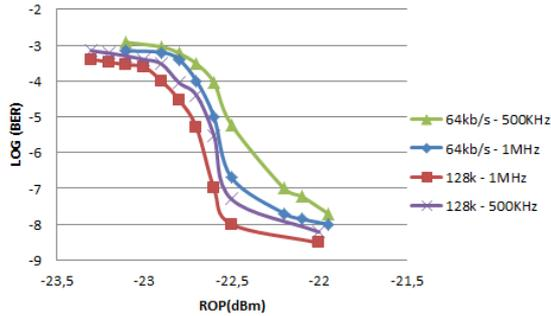
Fig. 5: BER performance as a function of the received optical power
