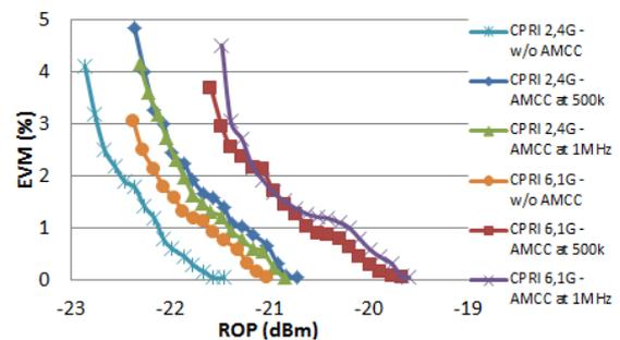
Fig. 4: EVM performance as a function of the Received Optical Power (ROP)
