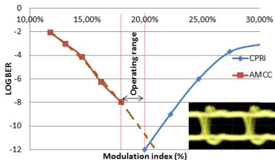
Fig. 2: CPRI and Pilot Tone BER performance for different modulation index and optical eye diagram at 20% modulation index
