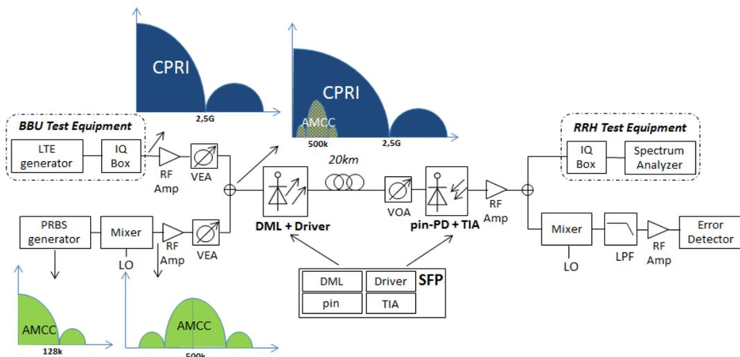
Fig. 1: Experimental setup
