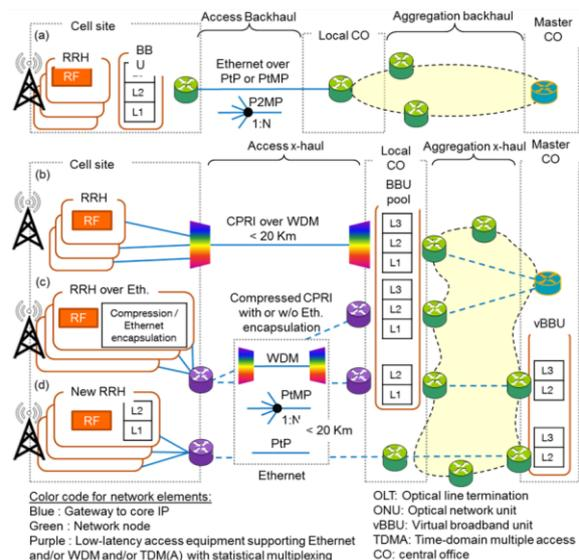
**Fig. 1:** (a) Existing mobile scenario, (b) CWDM C-RAN, (c) possible fixed-mobile convergent scenarios and (d) V-RAN.
