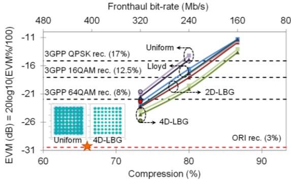
**Fig. 3:** EVM for different compressions and quantization techniques. 64QAM (●), 16QAM (■) and QPSK (▲).
