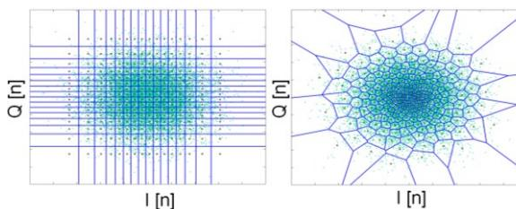
**Fig. 4:** 4 bits/sample comparison between scalar (left) and 2D vector quantization (right).
