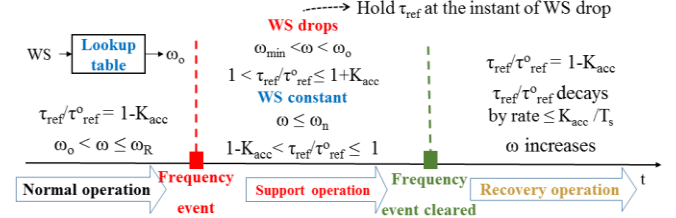
Figure 4. Illustration of the operation regions of Accelerative de-loading.
