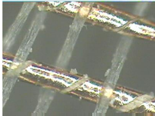
Figure 6: Micrograph of metallic organza
