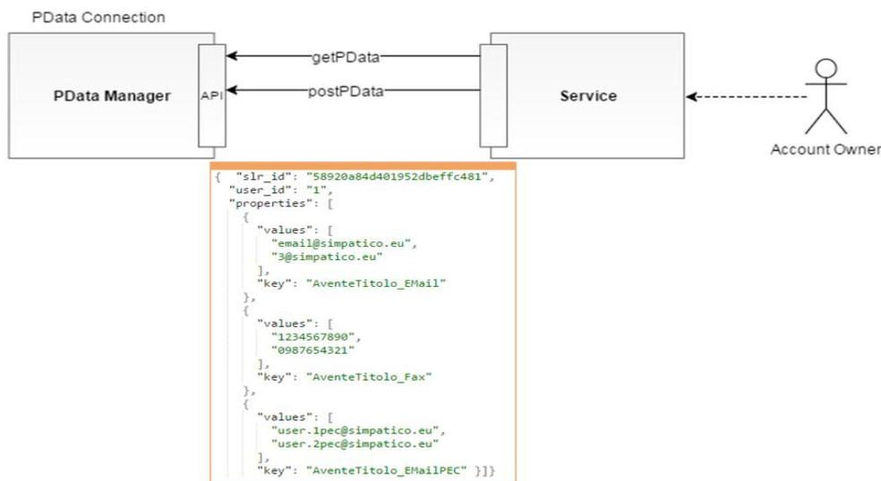
Figure 12 – PData Manager interactions with external service and related message exchanged
