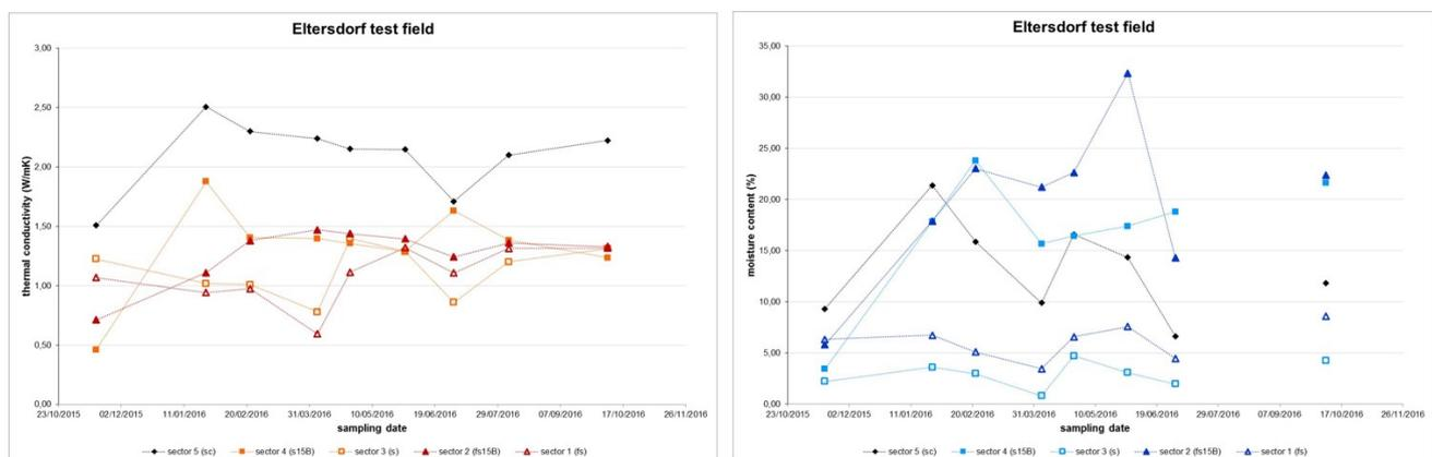
Fig. 1: Thermal conductivity and moisture content determined monthly on five different soil mixture in the ITER test site in Eltersdorf.
