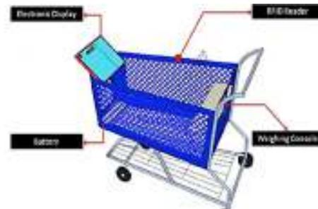
Fig.4: figure shows Smart Trolley using RFID
