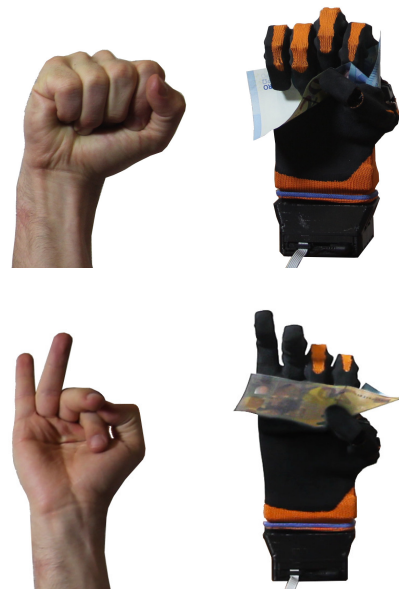
Fig. 9. An example of power and pinch grasp of a banknote. The similarity between the posture of an operator's hand and the Pisa/IIT SoftHand 2 highlights the effectiveness and the simplicity of this control strategy.
