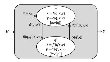
Figure 3: Graphical representation of open hybrid automaton.
