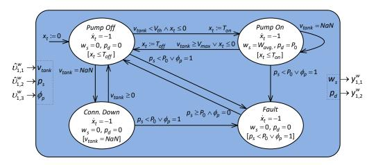
Figure A.17: Open hybrid automaton for the water pumping station.
