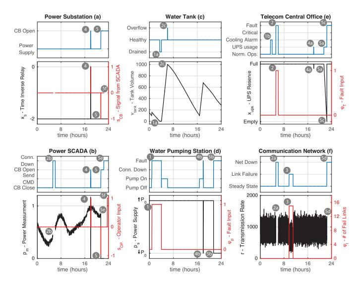
Figure 12: Plots showing the simulation of faults events for each component associated with the timeline in Fig. 11. For each component we show a plot with discrete state over time and a plot with what is best for each scenario, such as input/output variables and/or continuous state over time.
