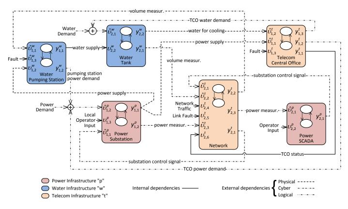
Figure 8: Model composition of CIS components.
