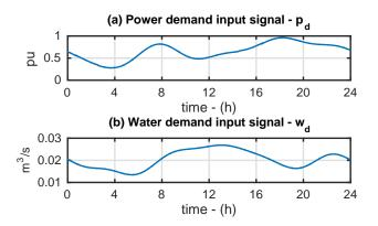
Figure 10: Profiles of input signals for power demand  $(p_d)$  and water demand  $(w_d)$  for all simulations.
