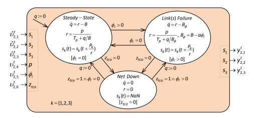
Figure B.19: Open hybrid automaton for the telecommunications network.
