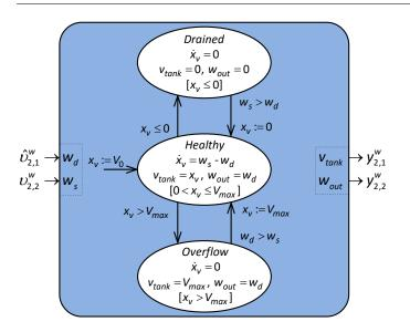
Figure A.16: Open hybrid automaton for the water tank.
