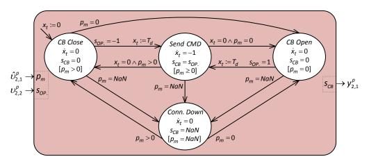
Figure 7: Open hybrid automaton for the power SCADA.
