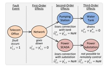
Figure 9: Example of n-order cascading effects due to dependencies, after a fault in the telecom central office.
