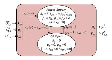
Figure 6: Open hybrid automaton for the power distribution substation.
