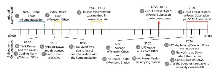
Figure 11: Simulation timeline with induced events/faults at the top and their subsequent consequences at the bottom.
