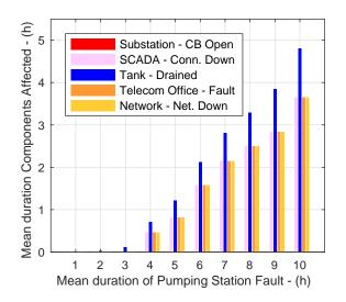
Figure 13: Plot showing how the duration of a water pumping station fault affects all the other CISs components.
