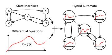
Figure 1: Hybrid automata integrate state machines and differential equations in a single formalism with uniform mathematical semantics.
