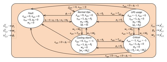
Figure A.18: Open hybrid automaton for the telecom central office.
