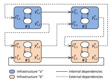
Figure 4: Composition example of open hybrid automaton models of CISs components with the notation for input and output variables.
