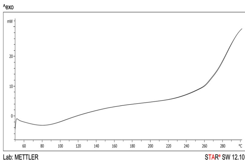
**Fig. 2: DSC thermogram of *I-hydrocel*.**
