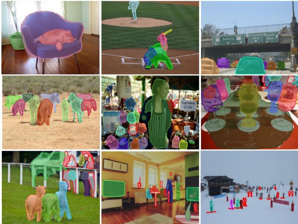
Figure 6. DeepMask proposals with highest IoU to the ground truth on selected images from COCO. Missed objects (no matching proposals with \text{IoU} > 0.5 ) are marked with a red outline.
