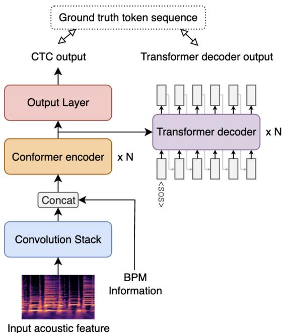
Figure 2. Overview of our proposed model architecture.
