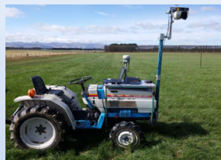
Tractor with LiDAR, GPS, and ruggedized laptop
