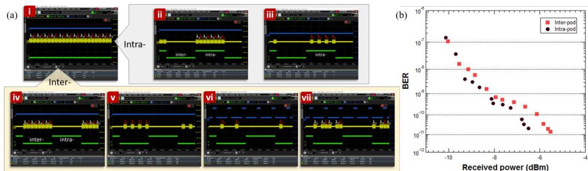
Figure 3: (a) Snapshots of NEPHELE packets in different spots of intra- and inter-pod communication. The red numbers (i)-(vii) corresponds to the same ones depicted in the experimental setup of Fig. 2; (b) BER vs. received optical power (optical modulation amplitude - OMA) for intra- and inter-pod scenarios.
