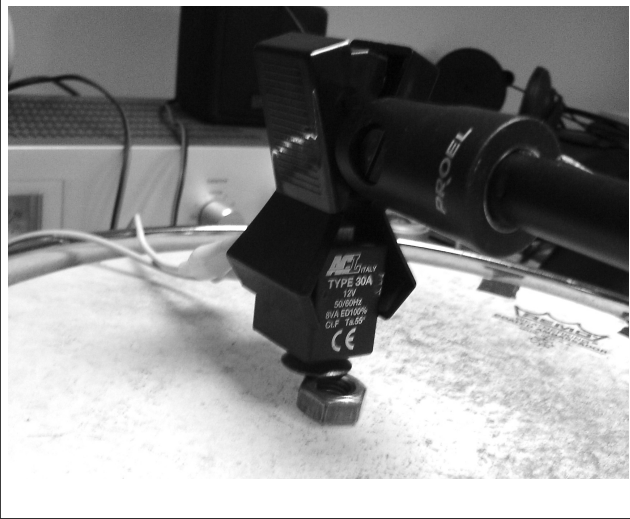
Figure 10. Testing a solenoid on a snare drum.
