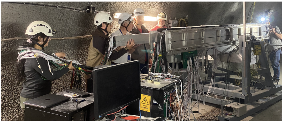
Figure 4: Insertion of a supermodule into the bar detector in PX56.
