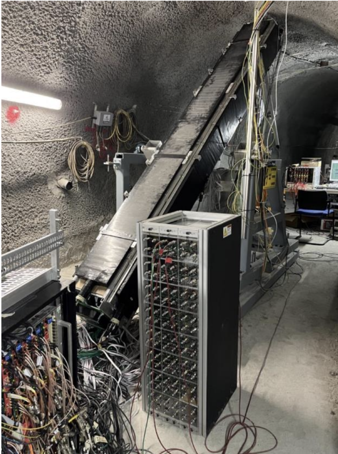
Figure 7: A photo of the completed bar detector pointing at the CMS IP in PX56.
