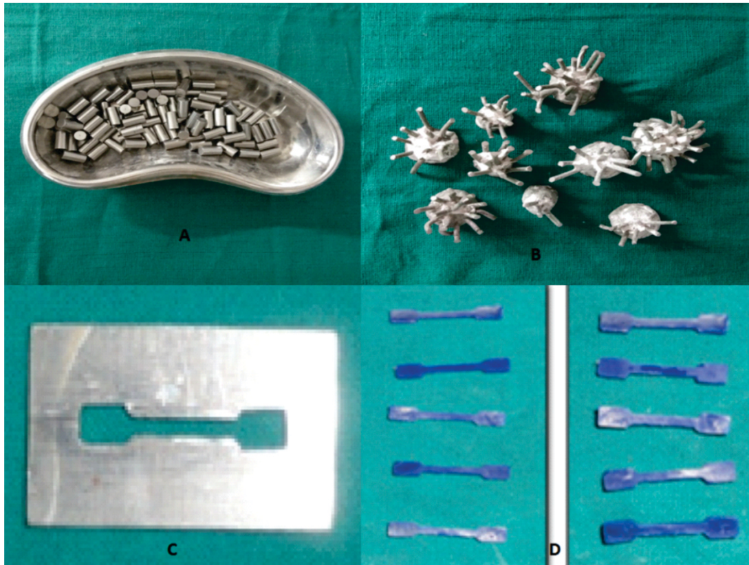
Figure 1: (A) New Alloy (B) Recast alloy (C) Mold for fabrication of test specimen (D) Wax Patterns of Specimen.
