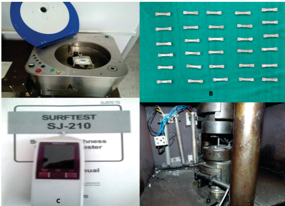
Figure 2: (A) Casting Machine (B) Cast Specimen of Alloys (C) Roughness Tester (D) Test of tensile strength.
