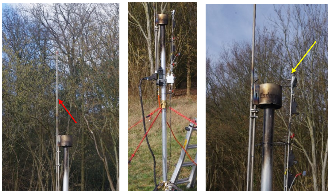
Figure 3: The burner of the flare with the suction pipe of flue gases (red arrow) and Figure 4 and Figure 5 The burner of the flare with the added spark igniter (yellow arrow).
