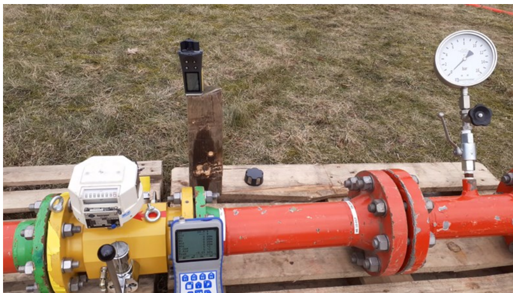
Figure 6: Flow meter (left, yellow), Pressure gauge (right), Anemometer (top centre), Flue gas analysis reader (bottom centre) in a single frame that was recorded by a camera.
