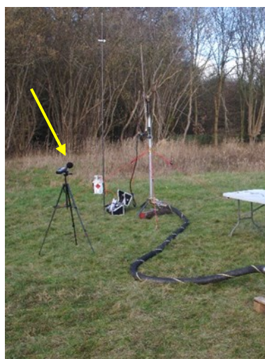
Figure 7: The Brüel & Kjaer sound meter and its position in the measurement setup (yellow arrow).
