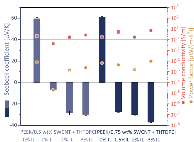
Figure 4. TE performance of PEEK/SWCNT composites (0.5–0.75 wt % SWCNT) without and with different amounts of ionic liquid THTDPCI.
