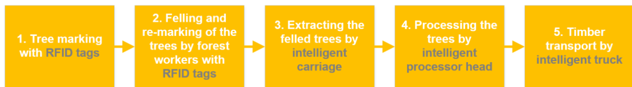
Figure 1. Flow chart: “Processes of the New Timber Tracking and Processing System”. The processes are highlighted in white, and the tools and machines in grey.
