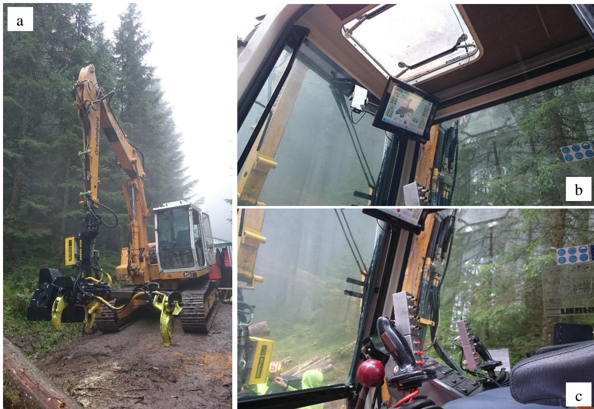
Figure 5. (a) Intelligent processor head on the Liebherr excavator. (b) System status display mounted at the top of the cab. (c) Processor head control units beside the joy sticks.
