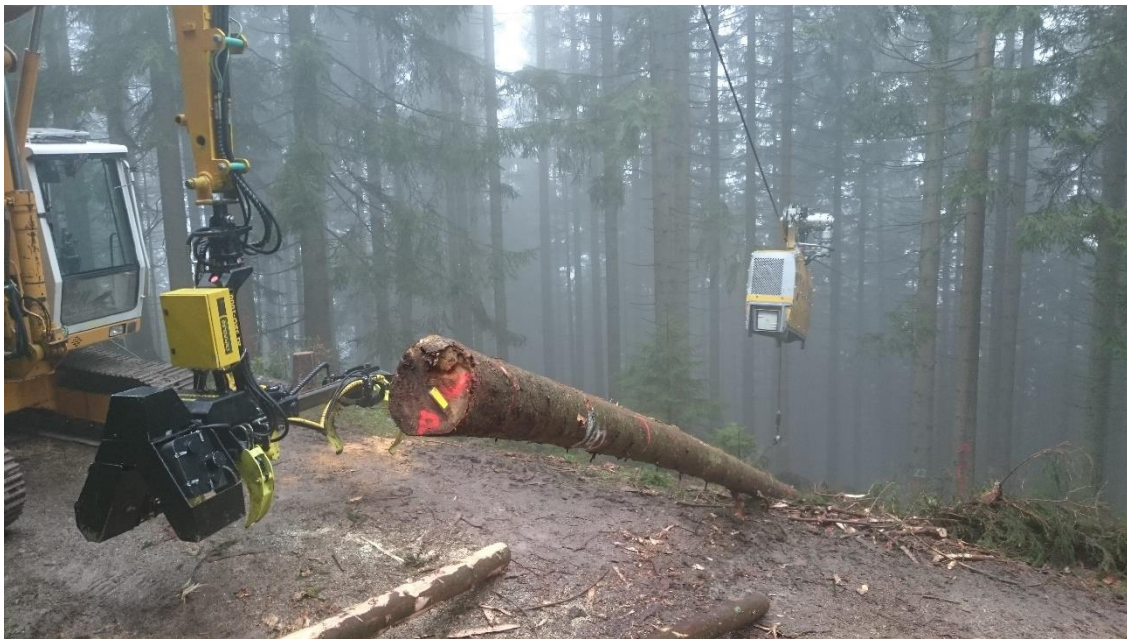
Figure 4. The intelligent carriage extracted and brought a tree to the excavator with an intelligent processor head in the landing area. RFID tag (yellow) visible on the bottom end of the tree.
