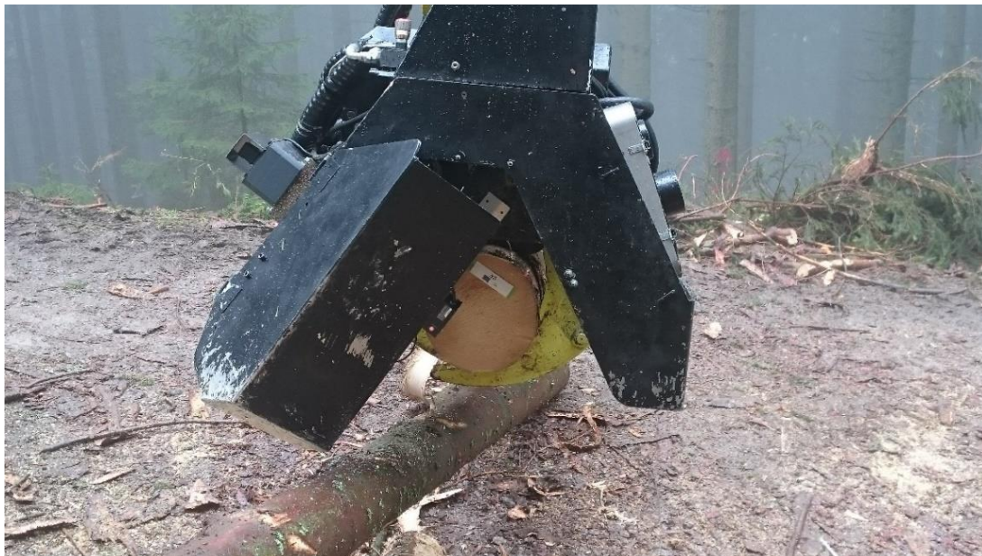
Figure 6. Stapling a new RFID tag (white) on the butt end of the log by an intelligent processor head.
