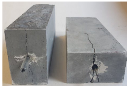
Figure 4: Concrete failure mode
