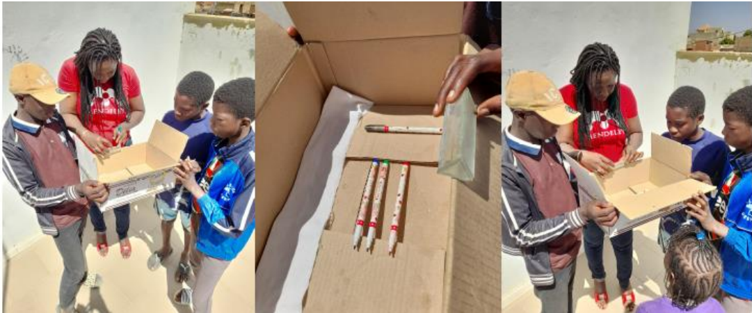
Fig. 1: First setup of the herschel's experiment with an artisanal prism in March 2021
