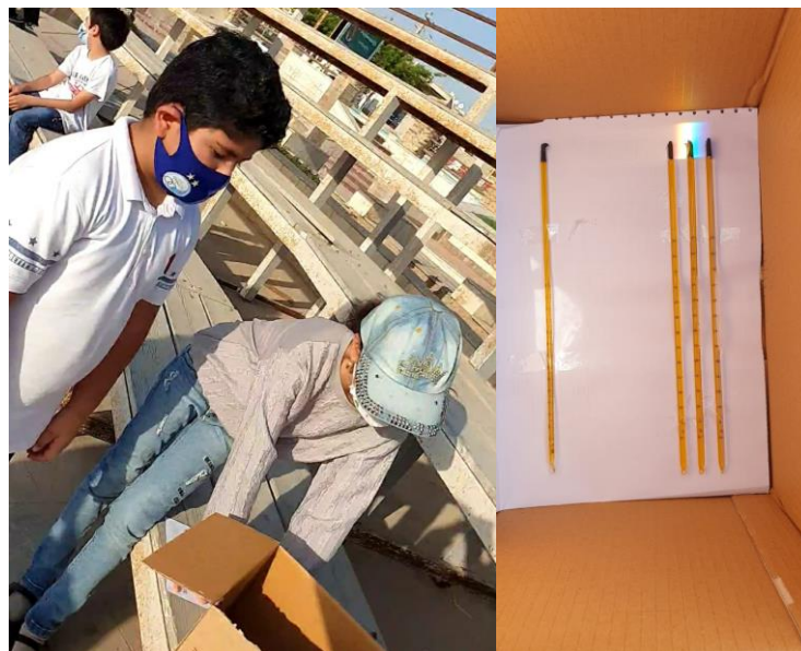
Fig4: Students are trying to find the infrared with termometers and a prism.
