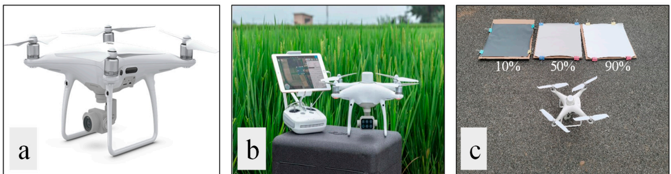
Figure 2. (a) UAS with digital camera for V images, (b) UAS with multispectral camera for V-NIR images, and (c) diffuse reflective plates.
