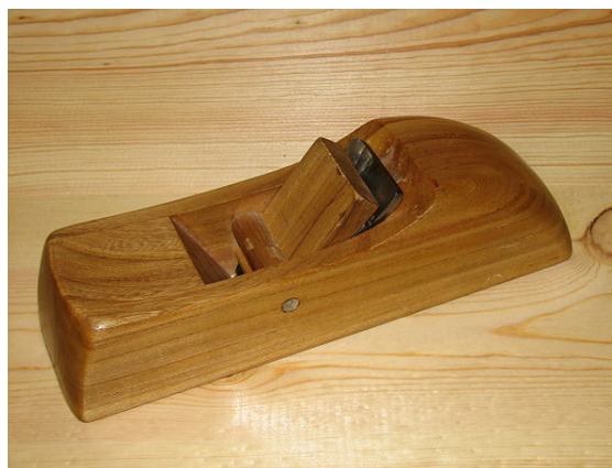
A wooden hand plane made of American elm.
