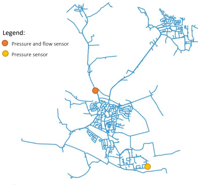
Figure 2-4 Location of measurement sensors in the Kapelle gas grid
