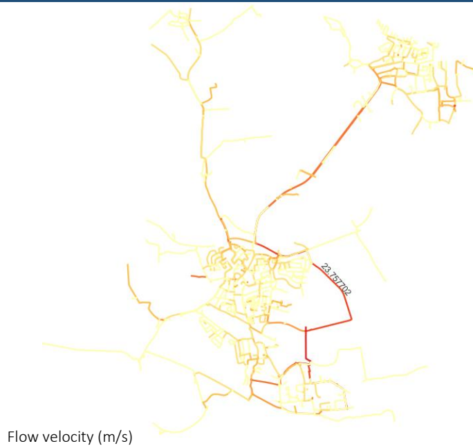
Figure 4-21 Flow velocity in the network for the new location of hydrogen delivery station.
