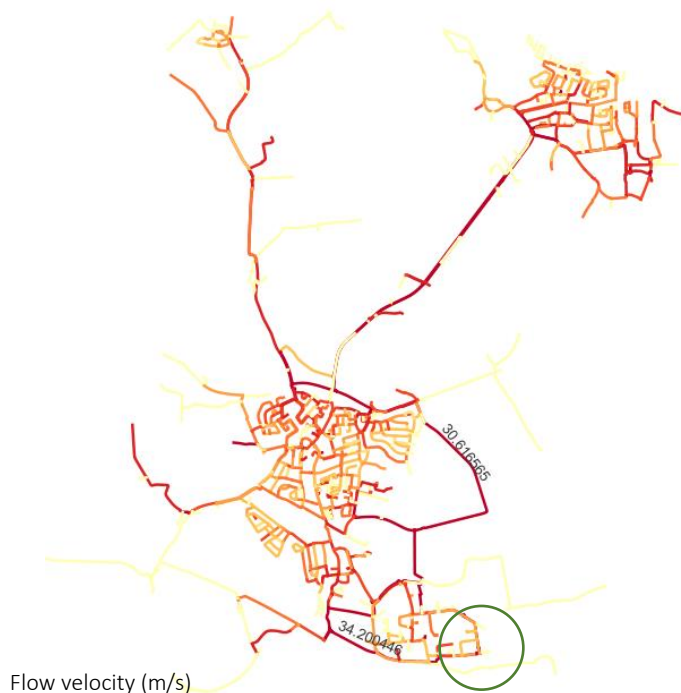
Figure 4-18 Flow velocity in the network for the hydrogen delivery station in the south east.
