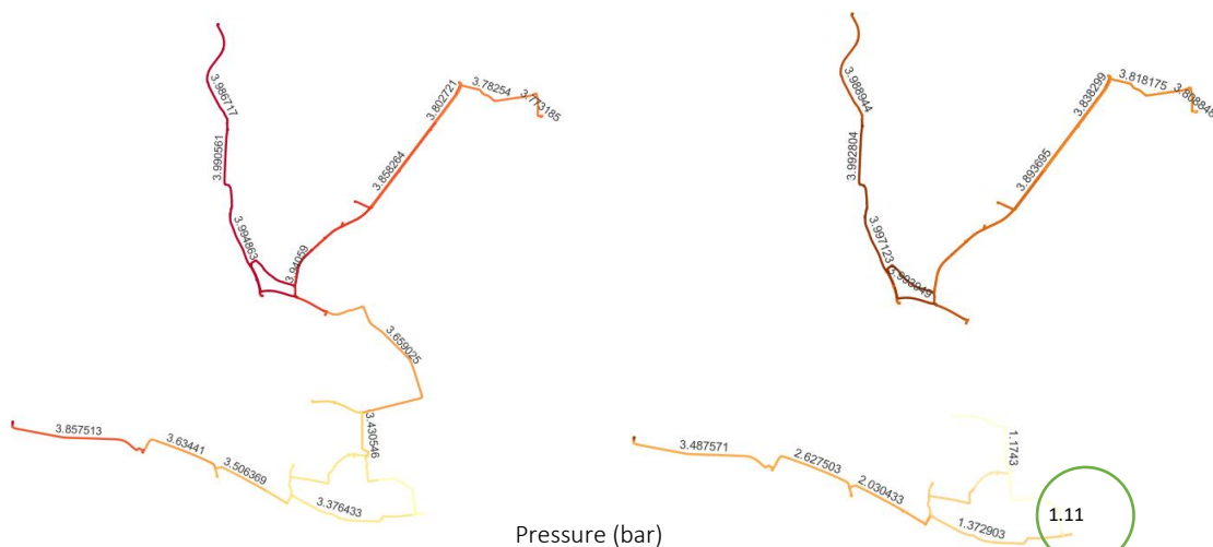
Figure 4-12 Comparison of pressure at 4 bar pipeline base scenario (left) and pipe break scenario (right)
