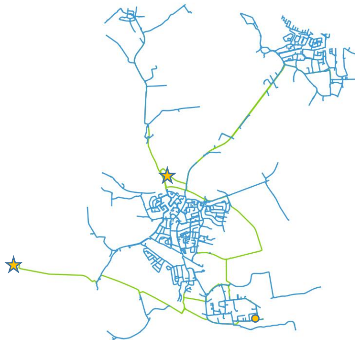
Figure 4-16 Location of the hydrogen delivery station (yellow circle) and the gas supplier 1 and gas supplier 2 is shut off (yellow star)
