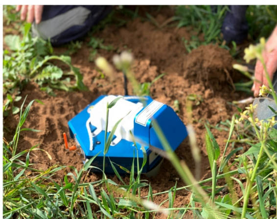
Figure 1. Picture of an installed Geode, along with the sensitivity of the Geode compared to commercially popular seismic nodes. Modified from Olivier et. al, 2022.
