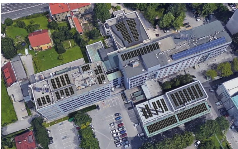
Figure 12 - Building of Faculty of Electrical Engineering at University of Ljubljana with existing PV installations (bluish modules) added predicted new PV installations (black modules).
