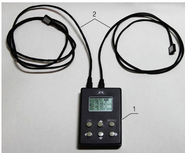
Fig. 2.1 Thermoelectric device for diagnosing inflammatory processes and pain syndrome in degenerative-dystrophic diseases of the Lumboischialgia: 1 – control unit; 2 – thermoelectric temperature and heat flow sensor
