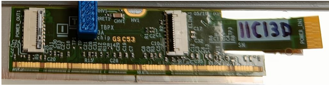
Figure 11: HDI 1x2 RD53A + 3D sensors
