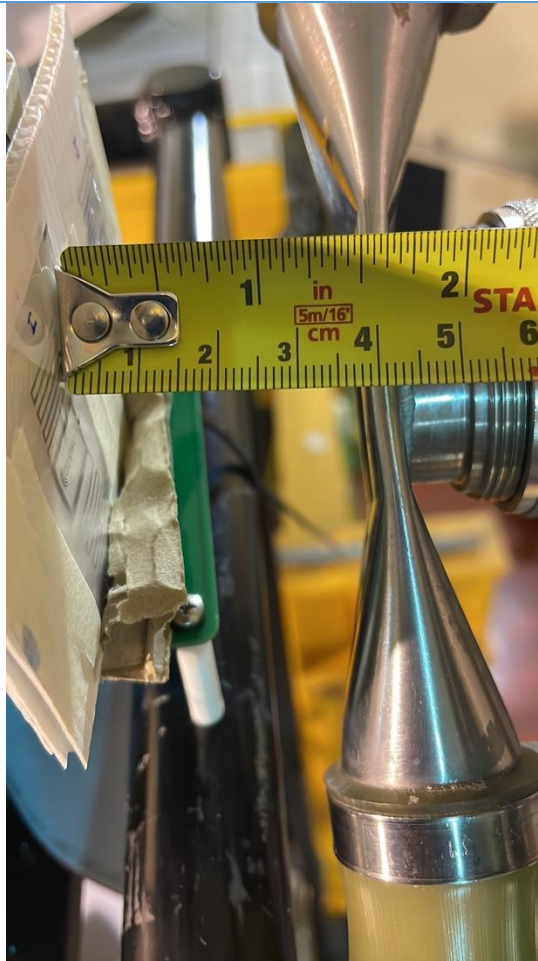
Figure 3: Detail of the neutron source and the distance from the tags.
