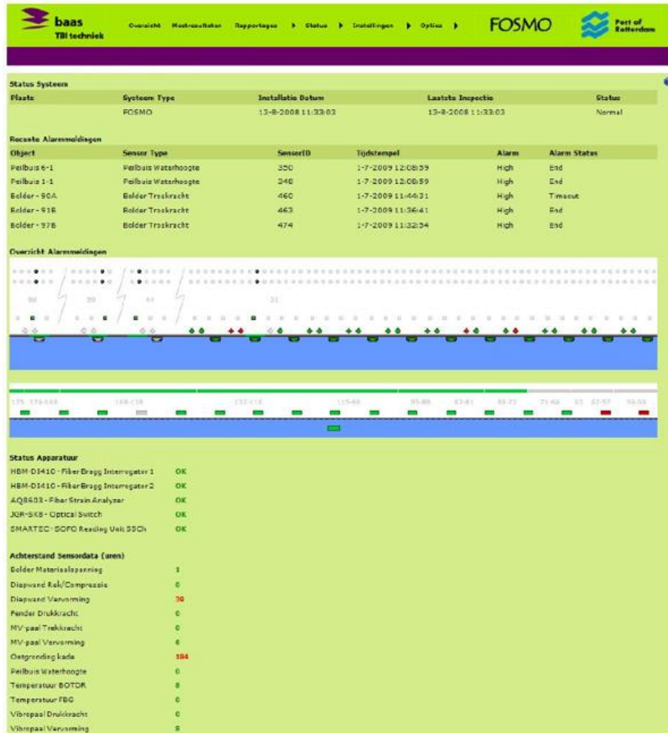
Figure 4.27: User interface of the FOSMO GUI (in Dutch), presenting the status of the instrumentation along the quay wall. Displayed is the working status of the data loggers (Status Apparatuur) and the correction function of the sensors, in terms of last measurement made in hours (Achterstand Sensordata (uren)).
