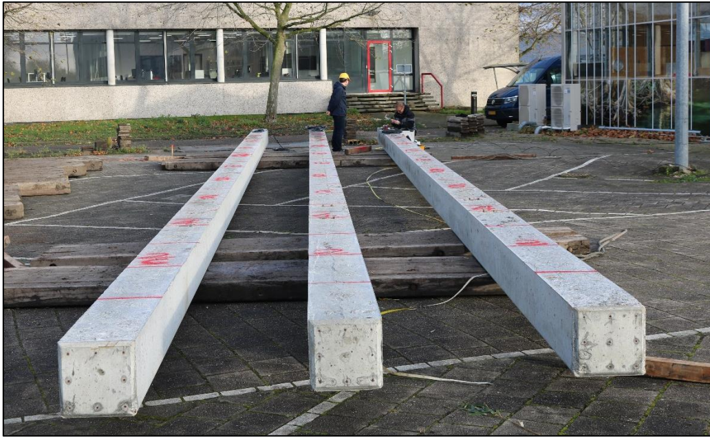
Figure 2.5: Driven precast piles lying on a site prior to installation so that a reference reading can be made. Following the initial reading, a second reading is made with the piles rotated 180° to compensate for bending effects between the two support beams
