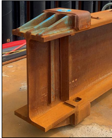
Figure 4.15: Picture of the widened tip at the base of an MV pile (Westerbeke, 2021)
