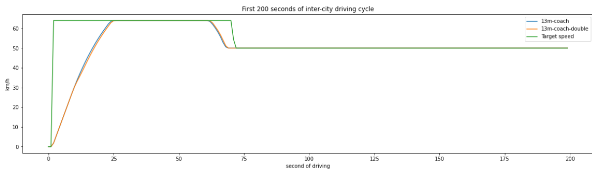
Figure 20 VECTO's Intercity driving cycle (first two hundred seconds)
