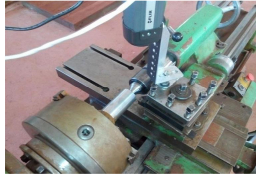
Fig. 4. Machining station with tool, specimen, and camera.
