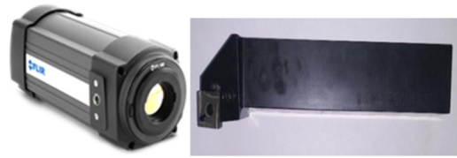
Fig. 3. Thermal camera FLIR A325sc and tool holder with the used insert.
