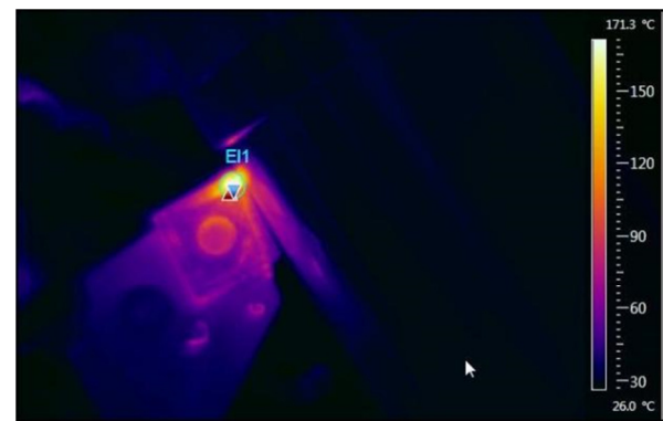
Fig. 12. Thermogram for V_c=78\text{m/min} , a=0.08\text{mm/rev} , and P=0.25\text{mm} .
