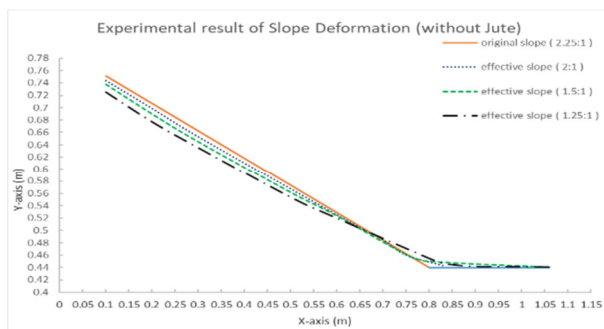
Fig. 5. Experimental results of saturated slope deformation without jute reinforcement.
