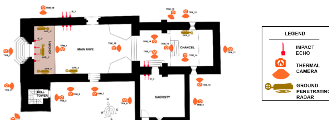
Figure 5. Non-destructive test locations (*for the tests in the Choir level)
