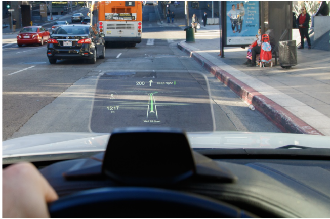
Fig. 5. Typical representatives of HUD ST optical - Hudway Drive [13]
