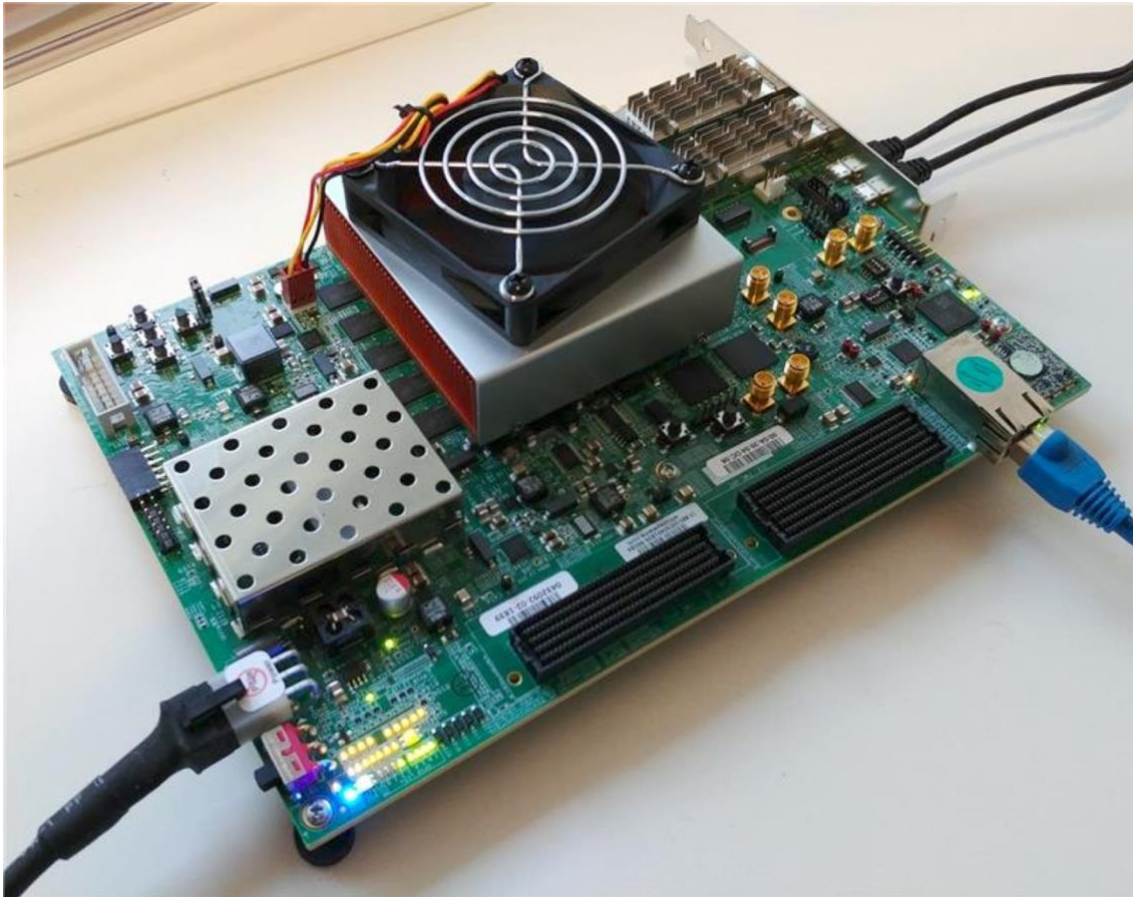
Figure 3.2: Xilinx Virtex UltraScale+ FPGA (VCU118 board) used to prototype the tile-based computer architecture for the M 3 OS at the circuit level
