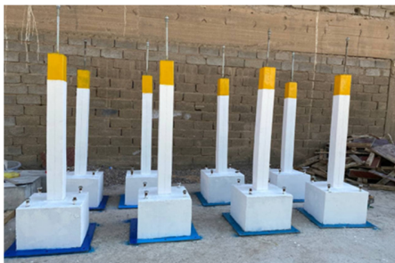
Fig. 5. The column models after casting.
