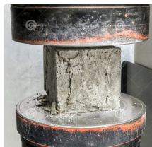
Fig. 2. Compressive test.
