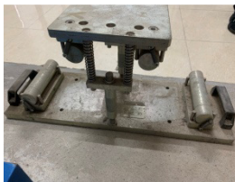
Fig. 1. Four-point bending test.
